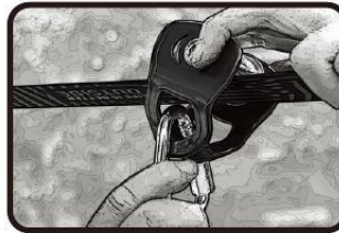
Attach Carabiner to Roller.
