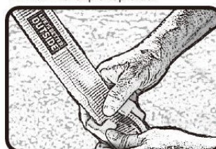
Squeeze Line fabric into gap in the Line Clip's top side.
